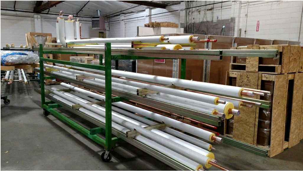
Finished racks ready for transport to jobsite
